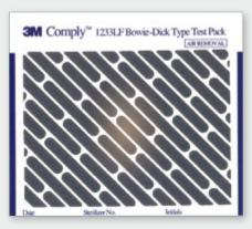
Bowie-Dick test sheet shows a non-uniform color change. Test sheet result indicates a small amount of residual air in the chamber.
