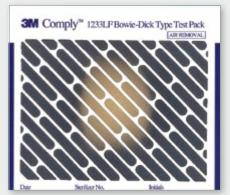
Bowie-Dick test sheet shows a non-uniform color change. Test sheet result indicates a large amount of residual air in the chamber.
